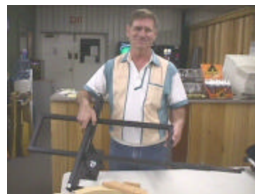
Earl Rutherford shows the boring handle and cage. Both of them are made from 1" square steel tubing. The long
