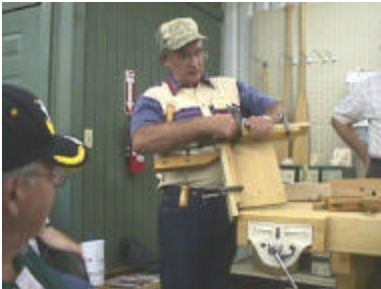
Jerry Shivers made a clamping jig to help him glue up mitered corners.
