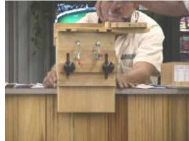
And a very adjustable mortise jig for his router
