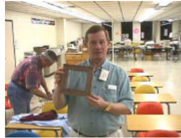
Rob Emanuel Showed us a jig he made to fit his table saw fence when cutting tenons and small pieces.
